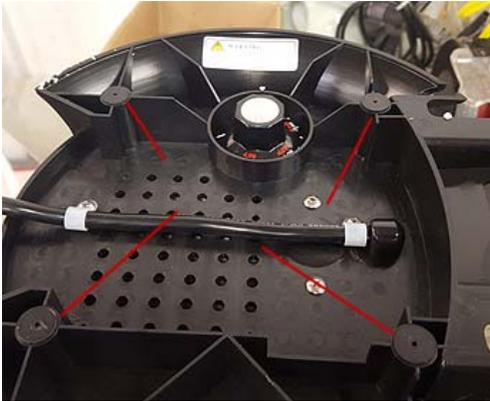
STEP 2: Remove Phillips screws under each foot using a Phillips screwdriver. Make sure when you replace these you do not overtighten them.
