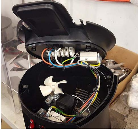
**STEP 4:** Do not spray while running. Spray only DIELECTRIC grease or lubricant into where the blue straw is pointing. Do not spray on electrical area. Only into metal shaft area. Let sit for up to four hours (or per product instructions). Test and replace base with screws. Repeat if necessary.
