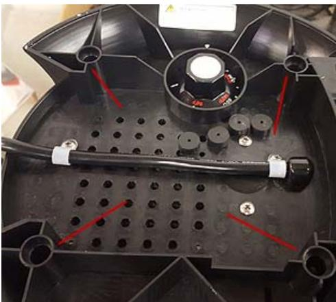
**STEP 3:** Gently remove the base. Do not disconnect any wires or pull on any wires. Having someone support this while you spray is recommended.
